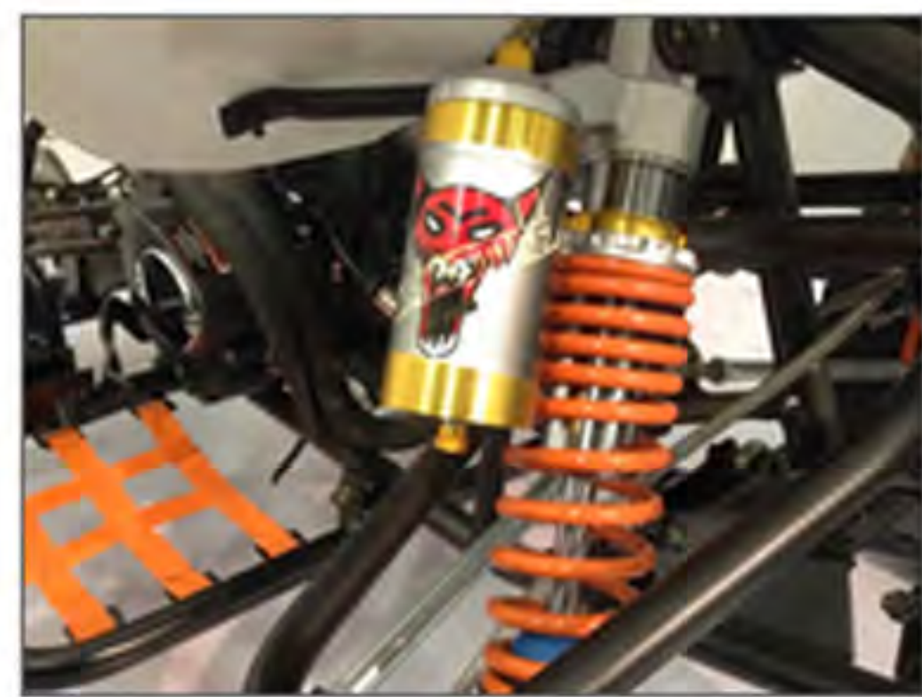
Adjustable Nitrogen Filled shocks
