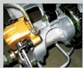
New Design Swing Arm Rear Hydraulic disc Brake
