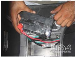
Connect the MAIN RED WIRE and RED WIRE with FUSE to the RED TERMINAL on the battery.
