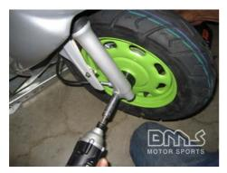
Attach the nut and tighten using 14 mm socket and crescent wrench
