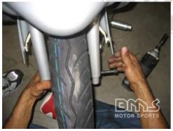
Insert the bolt through the wheel and fork assembly
