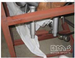
Remove the bolt, nut and spacer holding the front forks to the frame. DO NOT DISCARD the bolt nut and spacer.
