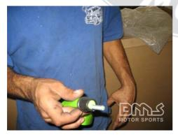
Install the rubber weatherproof seal on the end of one of the wing mirrors
