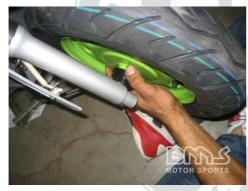
Attach the wheel bearing hub to the side of the wheel without the brake rotor.
