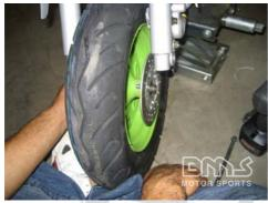
Insert the spacer into wheel on the side of the brake rotor.
