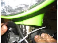
Insert the main bolt into the hole in the steering column and tighten using 14 mm socket and crescent wrench
