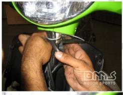
Remove the packaging from the front handlebars and slide the handlebars over the steering column
