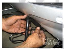
Install the kickstand by attaching the spring to the rear of the stand. Insert the bolt and tighten. Attach the other end of the spring to the notch on the unit
