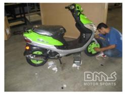
Remove the spacer from the front brake caliper
