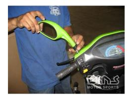
Screw the mirror onto the handlebars
