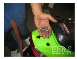
Remove the hex head bolts from the rear of the unit
