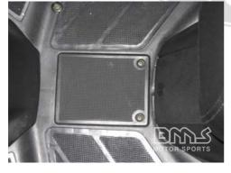
Reattach the battery cover using Phillips head screwdriver
