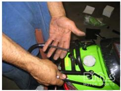
Position the rear rack over the holes in the rear of the unit and insert the bolts. There will be a longer third bolt for the rear-most hole
