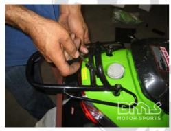
Tighten the bolts using the Allen wrench (provided)
