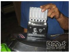
Attach Sulfuric Acid container to the tubes in the top of the battery
