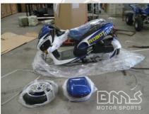
Remove the front wheel, trunk and seat from the unit.
