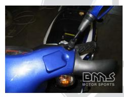
Screw the wing mirrors into each side and tighten the screw cap using a crescent wrench
