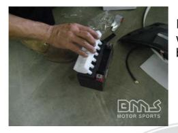
Remove Six Hole Funnel from plastic wrap and place into holes on top of the battery
