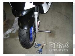
Insert the bolt removed earlier from the forks into the front wheel assembly from the side with the brake rotor and tighten.
