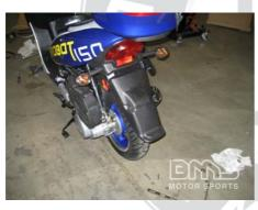
Attach the rear mud flap using the other 2 silver screws
