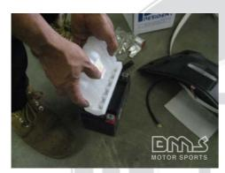
Attach Sulfuric Acid container to the tubes in the Six Hole Funnel
