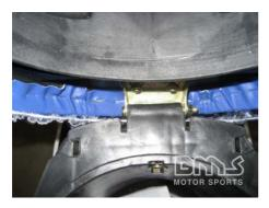
Slide the hinge bolt into the hole and bracket and tighten.
