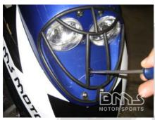
Remove the front screw under the headlight assembly using a Phillips screwdriver
