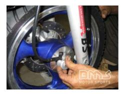
Place the spacer between the brake rotor assembly hole and the fork. Place the bearing assembly (hanging) on the side of the wheel without the brake rotor.
