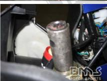
NOTE the notch at the back of the steering column
