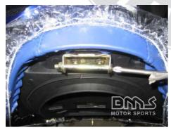
Unscrew the hinge bolt from the front of the seat using a Phillips head screwdriver. Line up the hole in the seat with the mounting bracket on the unit.
