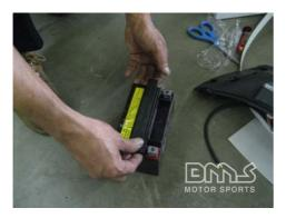
Remove Six Hole Funnel and cap battery holes with the battery hole plug strip.
