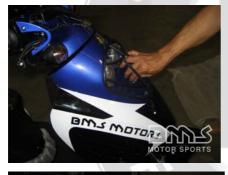
Replace the front screw and tighten using Phillips head screwdriver
