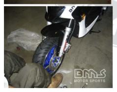
Slide the front wheel into the front forks
