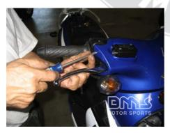
Remove the screws located on the upper and lower side of the handlebars. Repeat for both sides.
