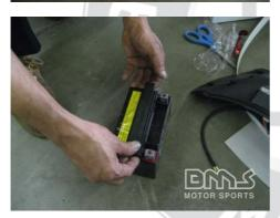
Remove Sulfuric Acid container and cap battery holes with the battery hole plug strip.
