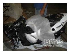
Remove the front cowling, front wheel, and front fender from the center of the unit.
