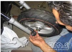
Insert the bearing assembly into the wheel in the side without the brake rotor
