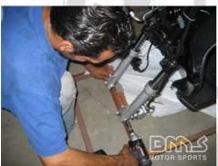
Remove the front bolt from the front forks. Do not discard this bolt, spacer, and nut.
