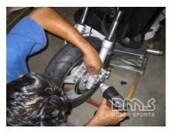
Remove the silver screws from the front forks. There are 4 screws
