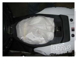
Open the seat to remove the items under the seat
