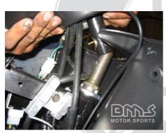
Line up the hole in the column with the hole in the handlebar shaft.
