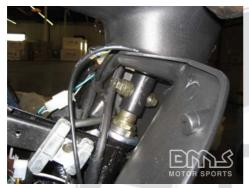
Insert the bolt and washer into the hole on the handlebar & steering column. Screw on the bolt and locking washer
