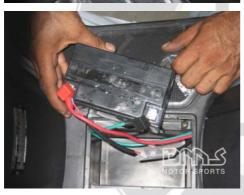
Connect the MAIN RED WIRE and RED WIRE with FUSE to the RED TERMINAL on the battery.
