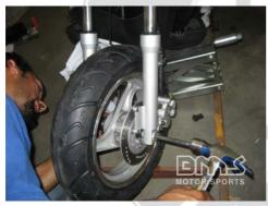
Align the front wheel and within the front forks and insert the bolt that was holding the unit to the frame. Using a hammer, push the bolt all the way through the hole
