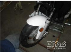
Attach the front fender with the shorter side to the front.
