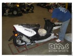
Attach the handlebars the steering column
