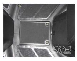
Locate the battery holder on the floor of the unit
