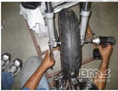
Using a 14mm socket and crescent wrench tighten the bolt and nut holding on the front wheel
