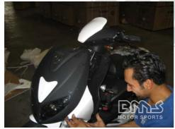
Attach the front cowling and line up the screw holes with the holes in the body
