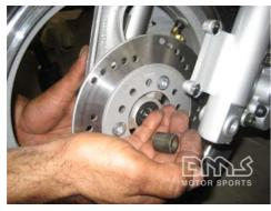
Remove the plastic spacer from the front brakes. Insert the metal spacer into the wheel on the brake rotor side.
