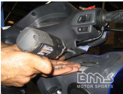
Remove the screws holding the front panel using a Phillips head screwdriver
