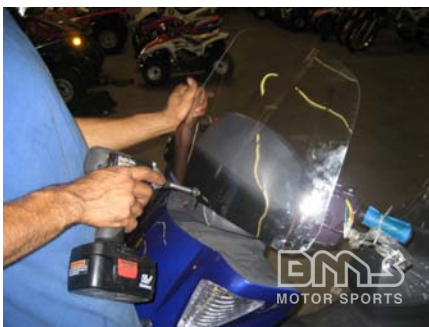
Attach the front windshield at the center bolt first
