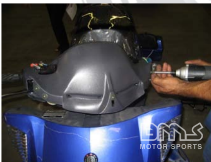
Remove the bolts that will be used to attach the front windshield using a 10 mm socket
