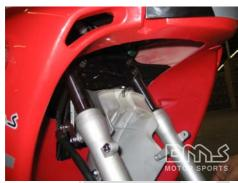
Locate and remove the bolt at the top of the fender mount using a 10 mm socket.
