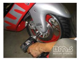
Attach the nut and tighten using 14mm socket.
