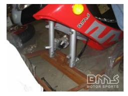
The bolt should slide out. DO NOT DISCARD the nut and bolt. This will be used to attach the front wheel.
