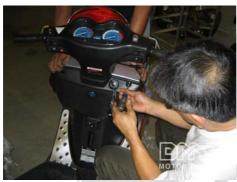
Screw the front cowling back on using a Phillips head screwdriver. There are 4 screws total.
