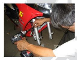
Remove the other 4 bolts from the front forks using 10mm socket. There are 2 bolts per fork.
