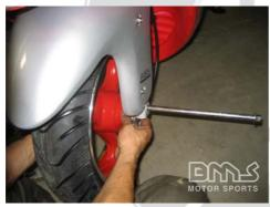
Insert the bolt removed earlier from the forks into the front wheel assembly from the side without the brake rotor
