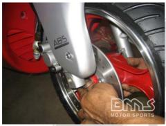
Insert the bearing spacer on the brake rotor side of the wheel.
