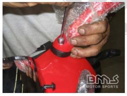
Place a washer onto the hex bolt and insert into the hole in the wing mirror assembly. Place one of the spacers under the wing mirror assembly onto the bolt and attach to the handlebars.
