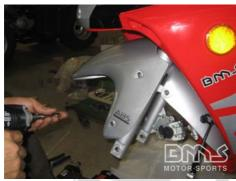
Attach the fender to the forks using 10 mm socket.
