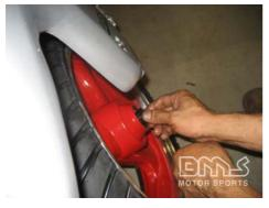
Insert the bearing assembly (hanging) onto side of the wheel without the brake rotor.
