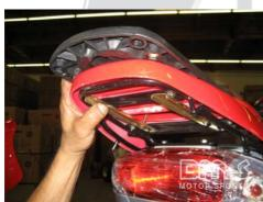
Rotate the adapter bars around and insert the remaining long screws into the top of the adapter plate
