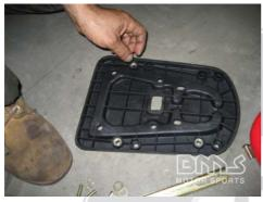
Remove the adapter plate from the storage compartment under the seat and located the mounting kit. The items in the kit are all gold in color. Insert the gold hexagonal nuts into the underside of the adapter plate.
