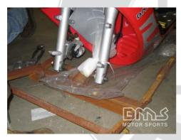
The front forks are attached to the frame by a bolt.
