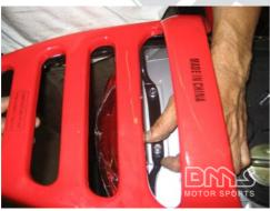
Remove the bolts from the top of the rear area using a 10 mm socket.
