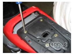
Using a Phillips head screwdriver and a 10 mm socket, tighten the screws
