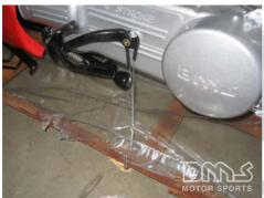
The rear of the unit is tied to the frame by wires. Untwist the wires and remove from the unit. If you have a pair of wire cutters they will work also.
