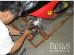
Loosen the nut and bolt using the 14mm socket.
