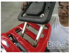
Slide the rear adapter assembly adapter bars into the second slot of the rear deck assembly.
