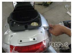
Remove the bolts on each side of the rear of the unit using the 12 mm socket
