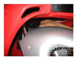
Attach the bolt to the top of the front fender using the 10 mm socket.
