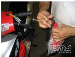
Attach the weatherproof rubber seal onto the end of the wing mirror assembly. Repeat for the other mirror.
