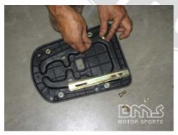
Flip the adapter plate over, making sure the screws do not fall out. Place an adapter bar onto the back of the adapter plate over each of the screws.
