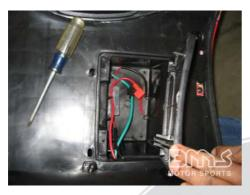
Open the battery cover using a Phillips head screwdriver
