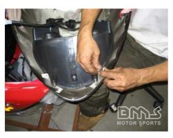
Attach the screw clips to the 2 tabs on the lower side of the front cowling. Make sure that the small hole is facing you as you attach them.
