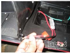
Connect the MAIN RED WIRE and RED WIRE with FUSE to the RED TERMINAL on the battery.
