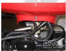
Thread the nut onto the other side and tighten using the 14 mm socket and the 14 mm Wrench
