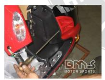
Remove the screws holding the front cowling using a Phillips head screwdriver. There are 2 screws. One on each side.
