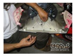
Attach screw clips to the 2 tabs at the top of the front cowling. Make sure that the small holes are away from you.
