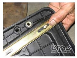
Attach the a nut to each of the screws but to not tighten them down. Thread them on for 2 to 3 turns
