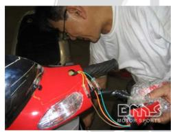
Connect the same color wires together. Connect the BROWN WIRE to the YELLOW WIRE
