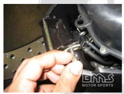
Using a 10 mm socket, remove the bolt holding the mounting bracket for the seat.
